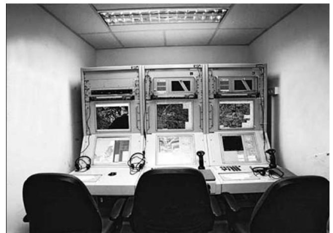
A Heron ground control station, which is staffed by an air vehicle operator (pilot) and a payload operator (navigator) [Photo: Department of Defence]
