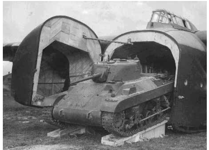
A British 'Hamilcar' glider unloading an M22 'Locust' tank [Photo: Imperial War Museum, London]
