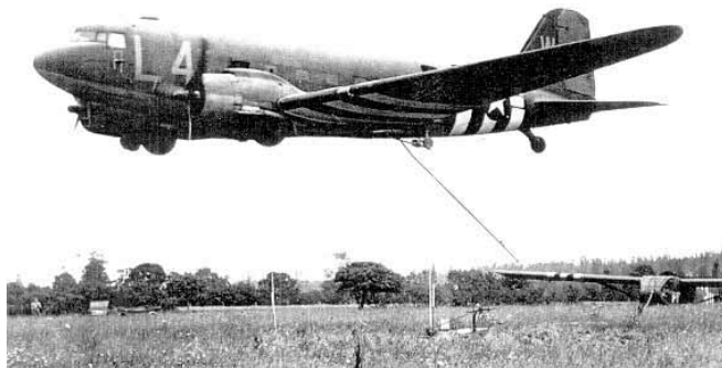
A ‘snatch’ of a Waco CG-4A by a C-47 [Photo: United States Army Air Force]
