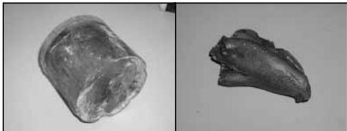
An explosively-formed projectile before (left) and after (right) detonation [Photos: Department of Defence].
