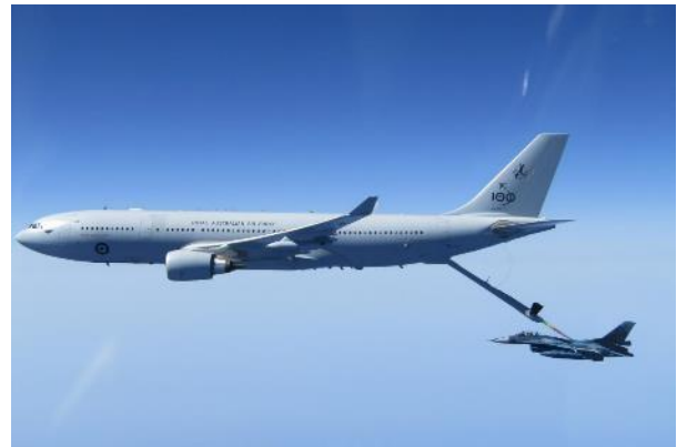
An air-to-air refuelling flight test between Royal Australian Air Force KC-30A Multi-Role Tanker Transport aircraft from No. 33 Squadron and Japan Air Self-Defense Force
