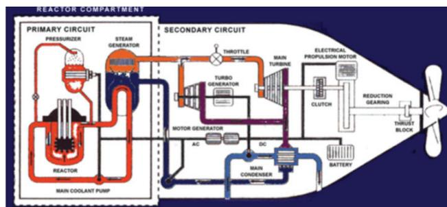
Figure 3: The submarine nuclear-propulsion plant – schematic. [Source: U.S. Navy undated]
