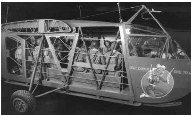
Cut-away of a United States ‘WACO’ CG-4A standard glider, which had two pilots and carried up to 13 personnel [Photo: Cradle of Aviation Museum, Garden City NY]
